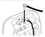
5. Route the adapter's cord through the narrow groove on the bottom of the bracket.
